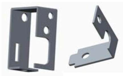
(b) Redundancy cable brace
