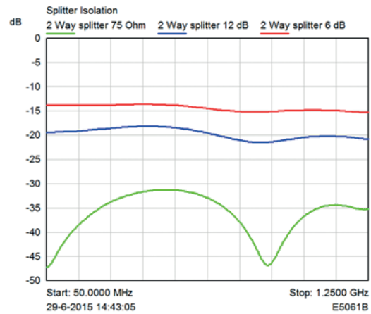
Fig. 7: Termination RL 6 dB isolation 2 \times (4 + 6) = 14 \text{ dB}
